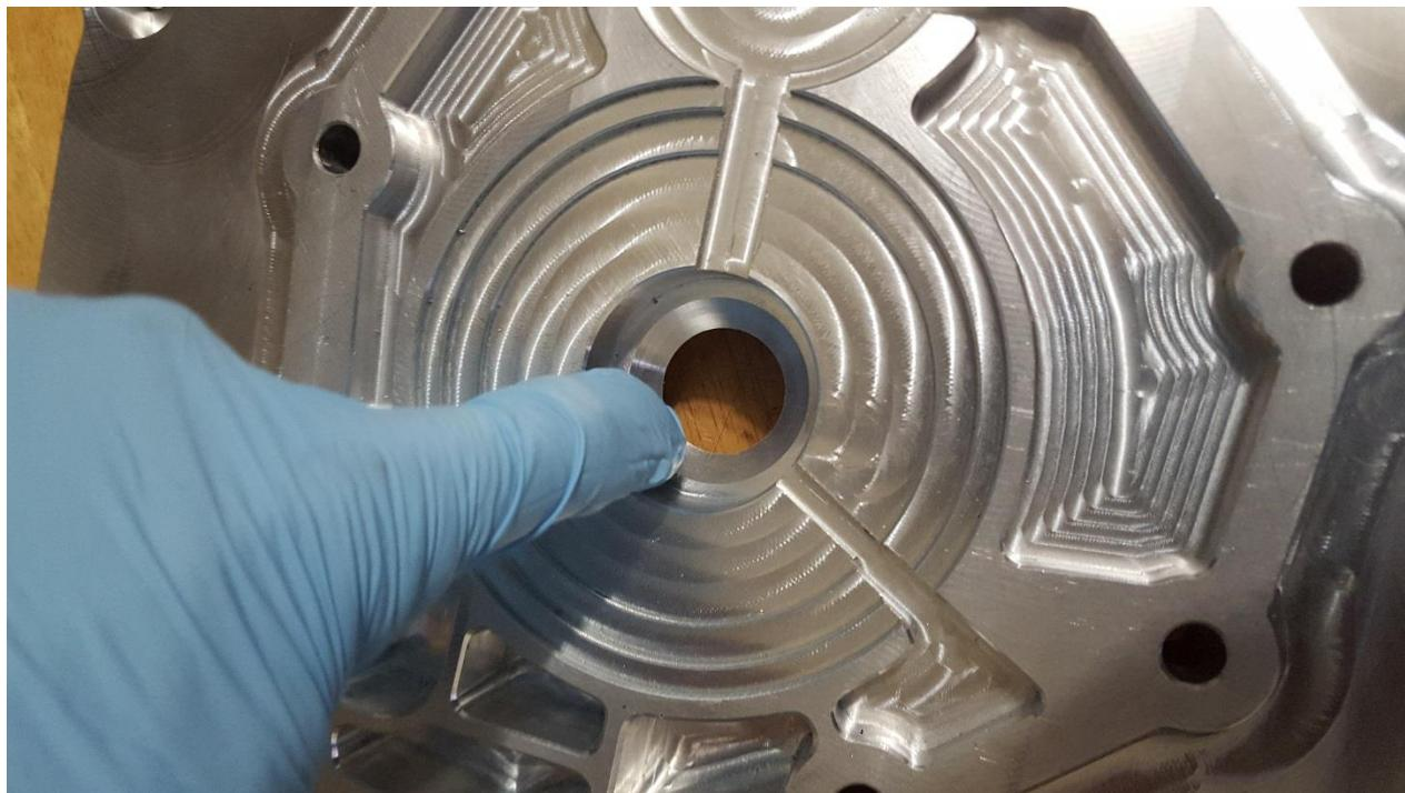
STEP 2: Remove the seal from the plastic wrapper, being careful not to rip or tear the outer edge. Once removed from the packaging, you will see a light amount of petroleum jelly on the inner most diameter of the seal (where the input shaft would ride). Take your finger and use some of this jelly to lubricate the outer most part of the seal, and inside gland of the adapter plate. This will help squeeze the seal into place with minimal force, and prevent tearing from rough edges.
