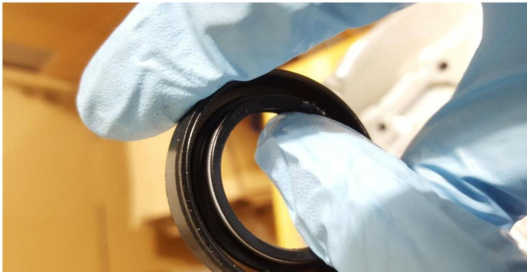
STEP 3: before installing the seal into the adapter plate, you will find two (2) machined channels that start from the center seal gland and go outward. These machined channels create very rough edges that tear the seal if the seal is not installed around those edges. Take care to place the seal in diagonally, so that when you start applying force to press the seal in, it does not get caught on the sharp edges of these machined grooves.
