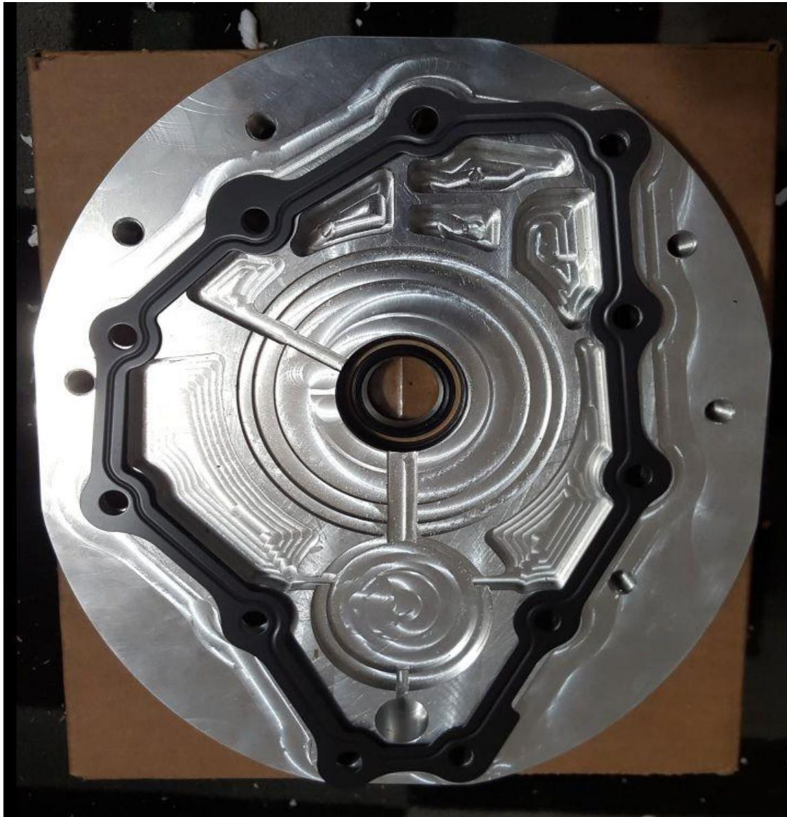
Make sure the liquid gasket is spread out evenly over the outlined surface, and the excess liquid gasket is cleaned off from the inner and outer edges.
