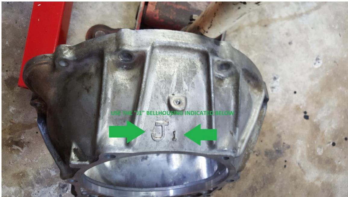
If you do decide to Use the "J3" bell housing, make sure to look on your adapter plate and verify that is Says "J3" on the Adapter plate where the bell housing mates with the adapter (it will be engraved very clearly on either side saying "J3"). This adapter plate is of a different thickness and will not work with the "J1 or J2" bell housing. (You have selected your specific bell housing in the drop-down menu).
