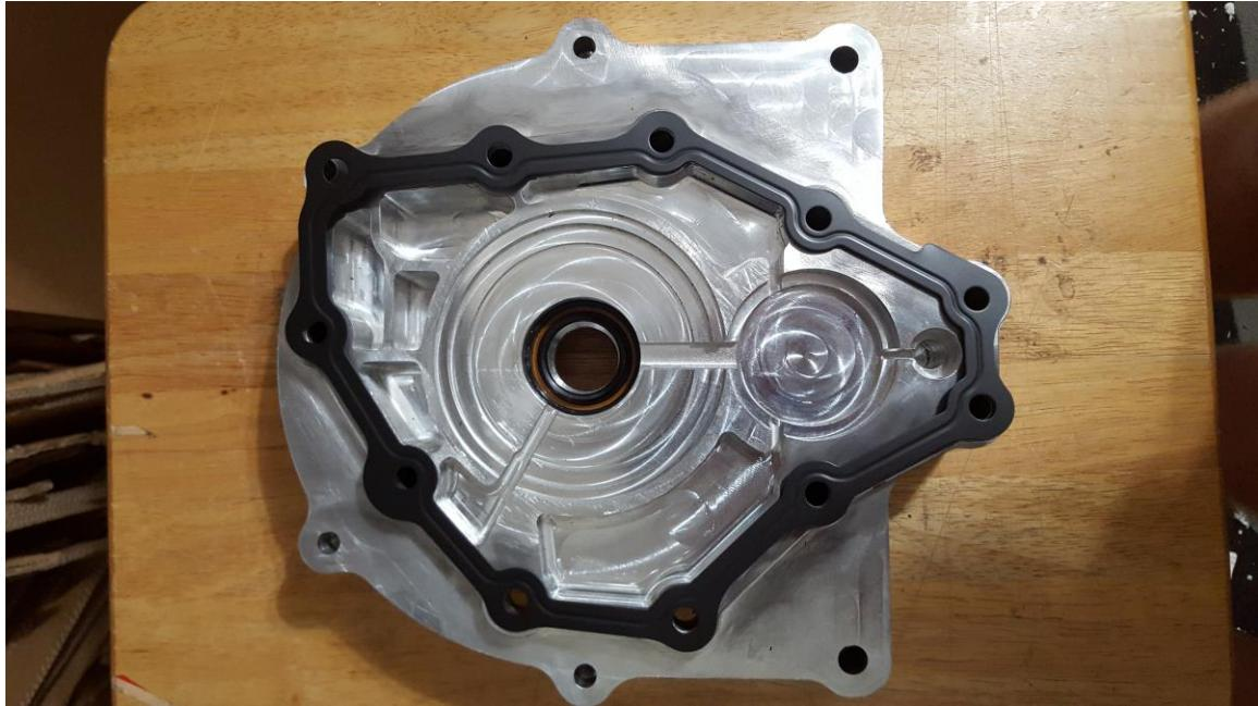
Make sure the liquid gasket is spread out evenly over the surface outlined in Black, and the excess liquid gasket is cleaned off from the inner and outer edges.
